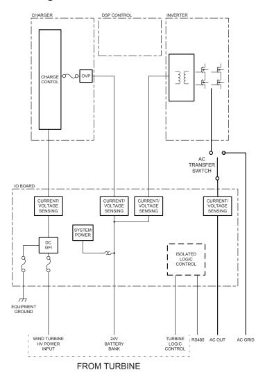
Figure 2.2 SMARTBOX™ Controller Diagram
